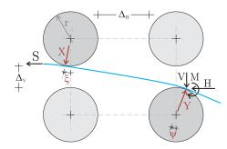
Figure 6: The scheme of the sliding sleeve constraint realized through two pairs of rollers.
