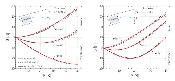
Figure 7: Comparison between experimental results (red curve) and the theoretical predictions. These have been reported for a perfect sliding sleeve (dashed curve) and for a sliding sleeve realized with rollers mimicking the experimental conditions (solid curve). Two rods have been used of external lengths 261 mm (left) and 424 mm (right) for different inclinations ( $90^{\circ}$ ,  $60^{\circ}$  and  $30^{\circ}$ ).
