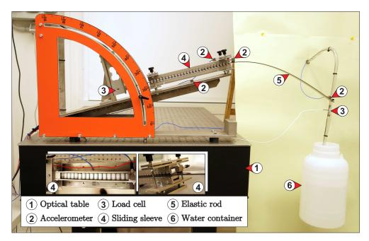
Figure 5: The test setup for the measure of the axial Eshelby-like force transmitted by a sliding sleeve, a realization of the scheme reported in Fig. 1.
