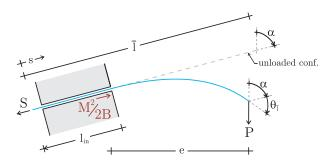
Figure 1: Structural scheme of the elastic system employed to disclose a Eshelby-like force. The elastic rod of total length  $\bar{l}$  is subject to a dead vertical load P on its right end, is constrained with a sliding sleeve inclined at an angle  $\alpha$  (with respect to the vertical) and has a axial dead force S applied at its left end. The presence of the Eshelby-like force  $M^2/(2B)$  influences the force S at equilibrium, which results different from  $P \cos \alpha$ .
